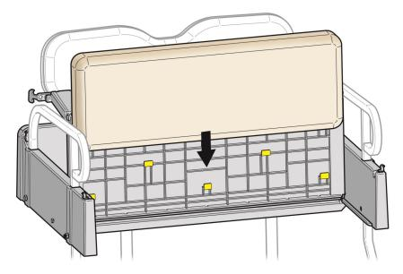
17. Lock the seat bottom into place with the (2) small retaining plates and (4) <u>M6 x 15</u> <u>Phillips Head Countersunk Screws</u> (**Bag #5**).
