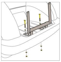
5. Loosely fasten the horizontal support brackets to the front seat back support brackets and vertical support bracket using (4) M10 x 30 Hex Head Bolts, (8) Flat Washers and (4) Nylock Nuts (Bag #2).
