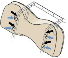
9. Remove the seat back support and the bag attachment assembly. Retain hardware.
