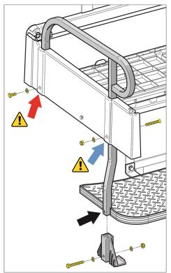
16. Slide the rear seat bottom onto the underside of the utility box deck until it clicks into place on the locking tabs (yellow).
