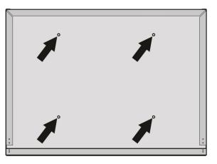
Fasten the latch catches to the tailgate using (2) <u>10-32 x 1" Pan Head Phillips</u> <u>Machine Screws</u>, (2) <u>Flat Washers</u> and (2) <u>10-32 Nylock Nuts</u> (black arrow).
