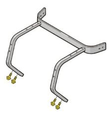
If reinstalling the factory top on carts with noncollapsible struts, cut the rear portion of the struts just inside of the rear most 90° bend. Remove any burrs with a file. Driver side shown.
